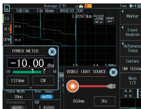
Example of multi-tasking with OTDR, optical power meter, and visible light source
