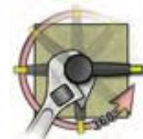
Using the 360° capabilities of the Swiveler®, the cable is positioned into desired orientation & temporarily hand tightened. Using a wrench, the hex nut is tightened to the recommended torque while holding the cable or connector in the desired location.
