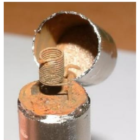
Figure 5-1 Internal Corrosive Damage
