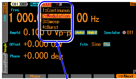
Set the oscillation mode to [Modulation]
