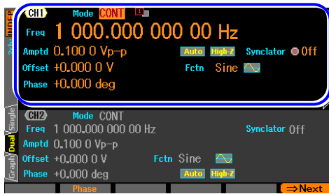
CH1 active (CH1 is the Setting target)
