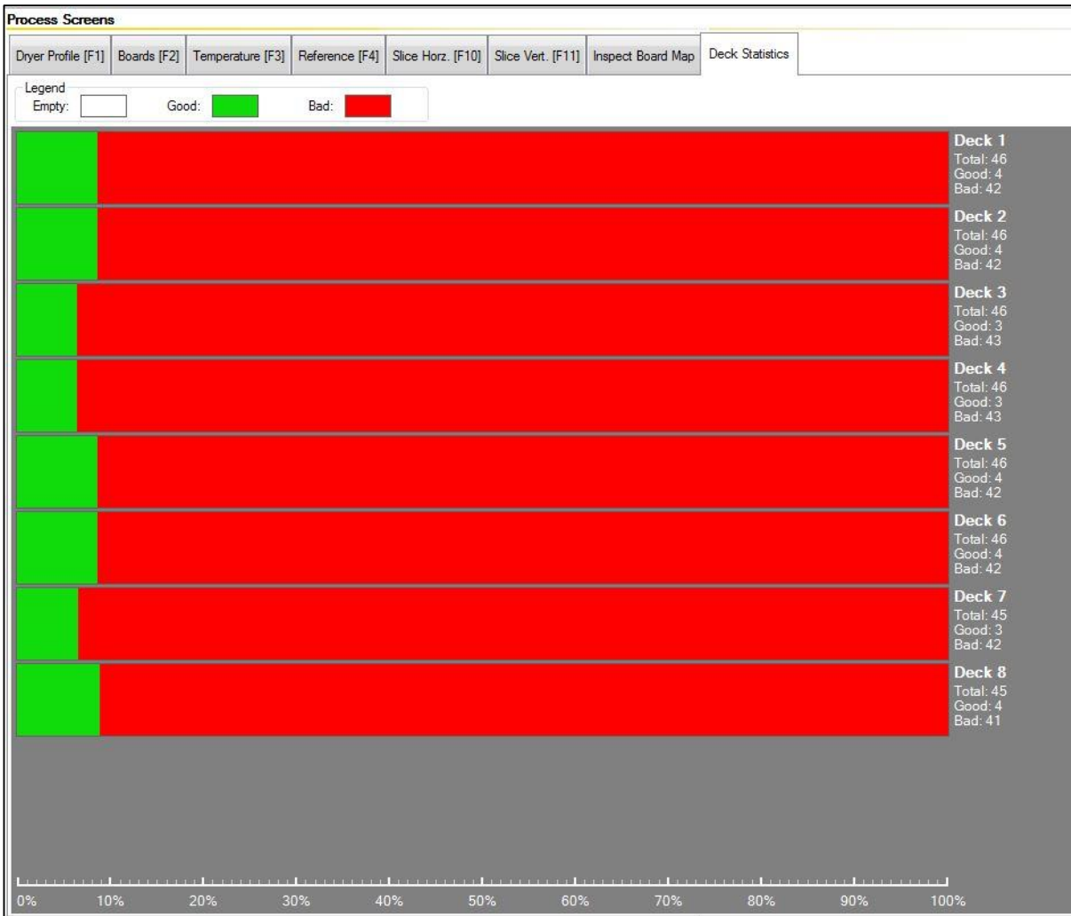
Figure 69: Deck Statistics Display shows the relation of good/bad produced wallboard sets
