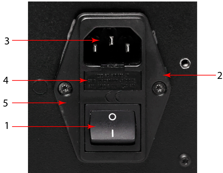
Figure 26 Power Supply Fuse Replacement
