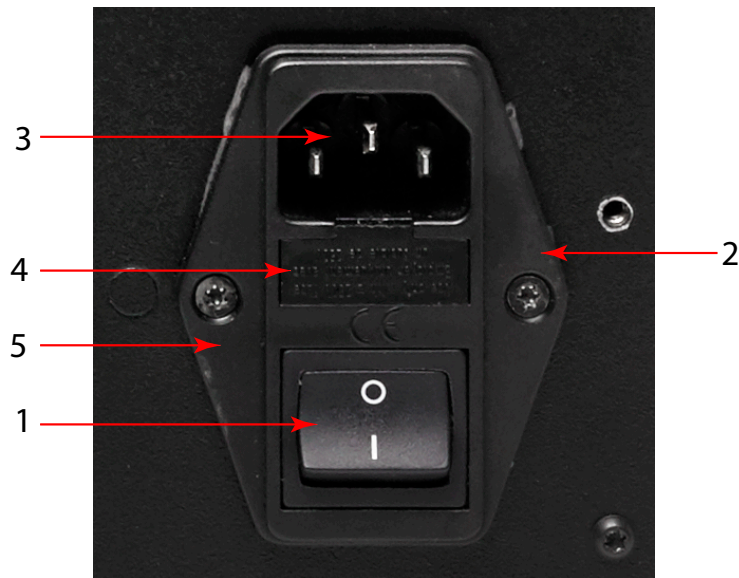
Figure 27 Power Supply Fuse Replacement
