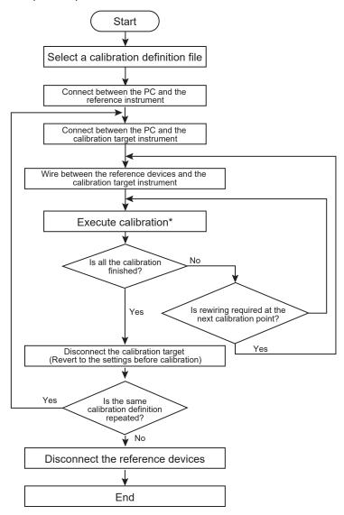
\*: When calibration is executed, the output of the reference instruments is turned on.
