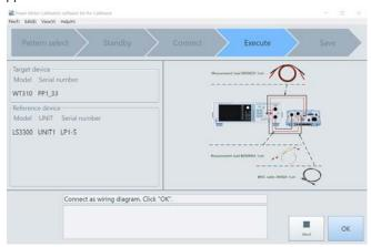
Confirm that the output of the reference instrument is turned off and connect wiring between the reference instrument and the calibration target instrument.
