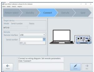
10. When Remote interface is set to other than "None", click Connect. The Connect button changes to the Disconnect button.
