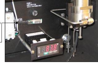
The runaway protection is provided by a J2 type device positioned between the temperature controller and the heater. This device cuts of power to the heater if the temperature inside the analysis unit exceeds 70°C. Should the J2 device cut power to the heater, correct the problem and reset the runaway protector device by exposing it to 0°C for a few minutes (a refrigerator freezer will do) or replace J2.
