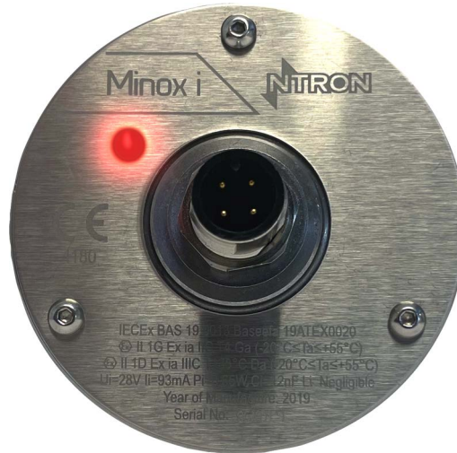
Figure 9. Minox i indicator LED
