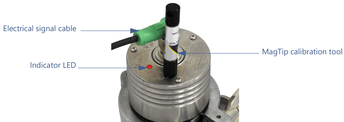
Figure 8. Minox i with MagTip calibration tool
