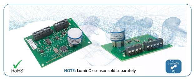
The LuminOx family (LOX) is a range of factory calibrated oxygen sensors which measure ambient oxygen partial pressure (ppO<sub>2</sub>) or volume O<sub>2</sub>% levels using the principle of fluorescence quenching by oxygen.
