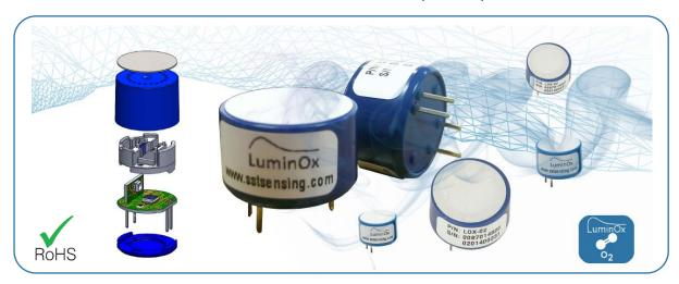
The LuminOx family (LOX) is a range of factory calibrated oxygen sensors which measure ambient oxygen partial pressure ( $ppO_2$ ) levels using the principle of luminescence quenching by oxygen.
