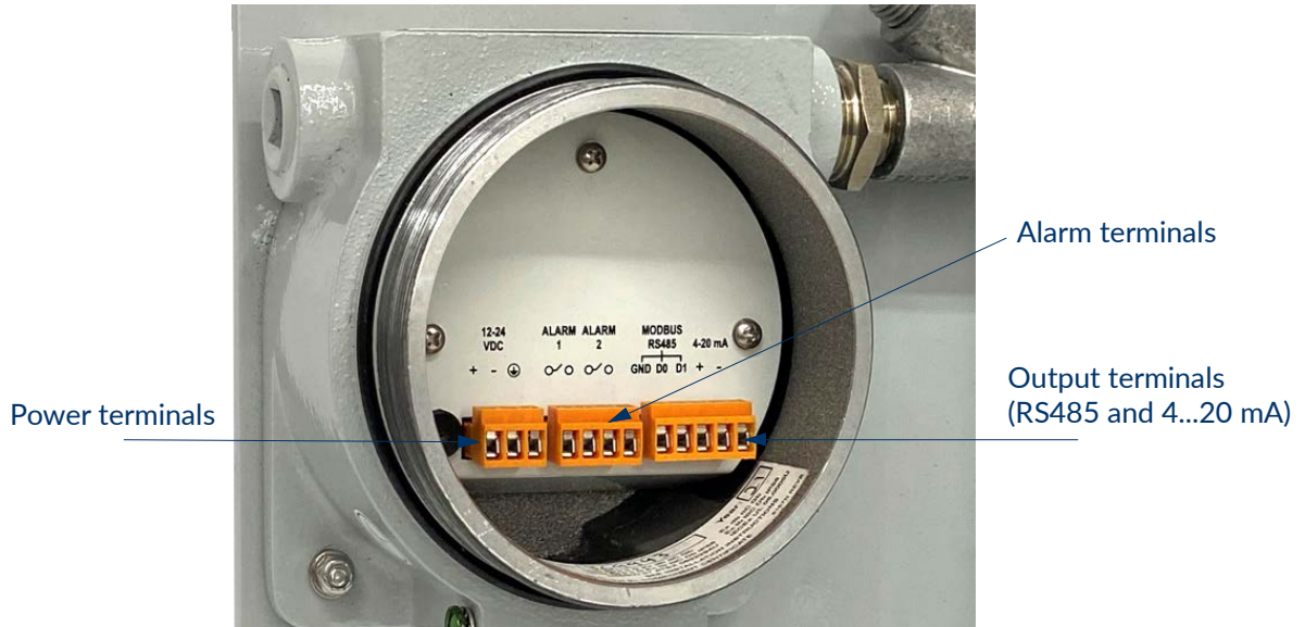
Figure 4. Wiring and connections (AIS models)
