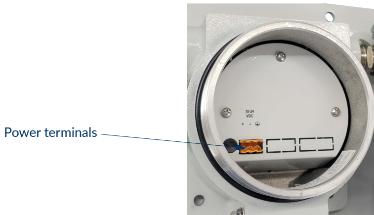
Figure 3. Wiring and connections (IS models)
