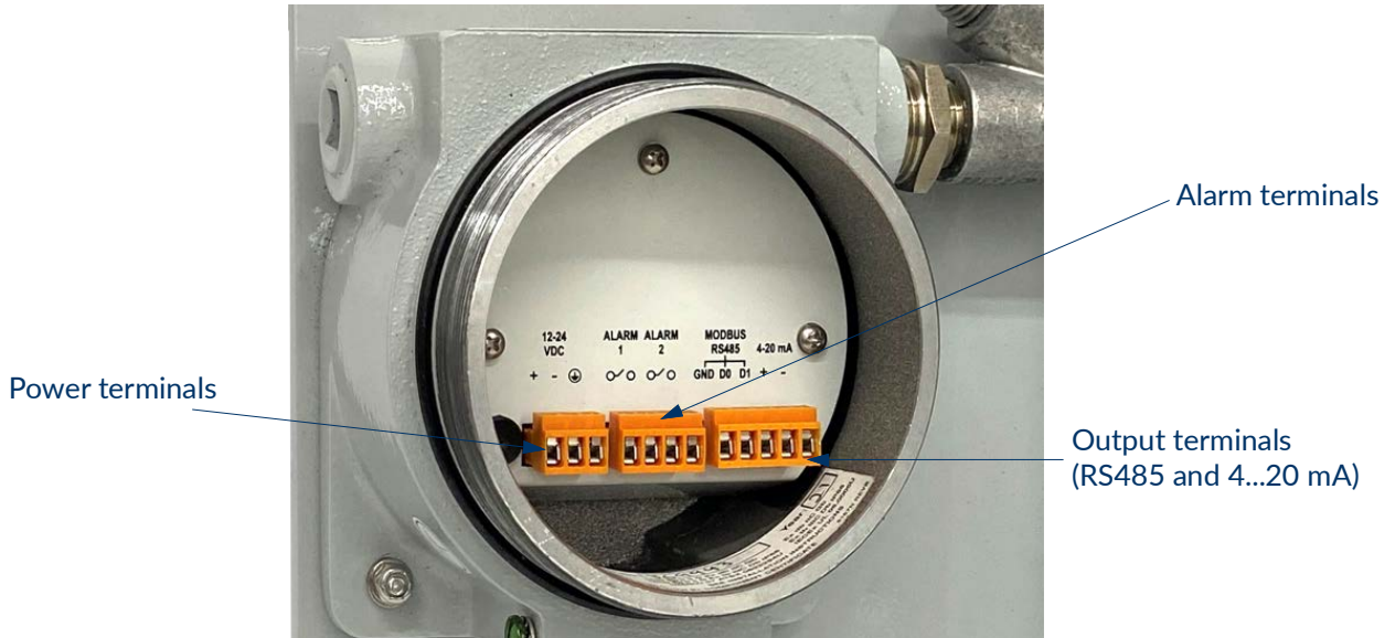
Figure 4. Wiring and connections (AIS models)
