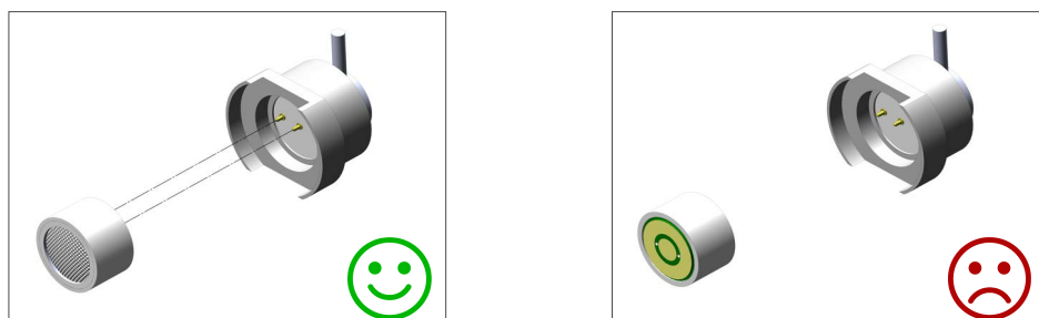
Figure 6. Aligning your sensor
