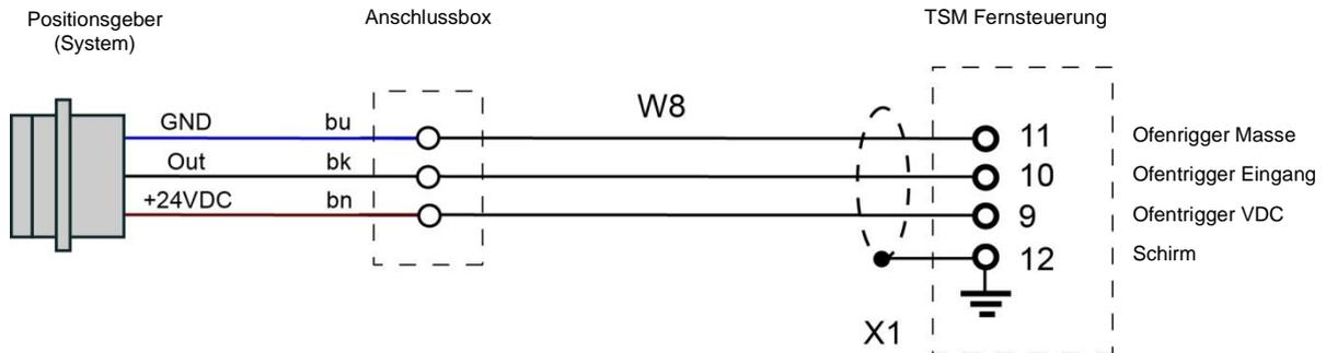
Abbildung 8-9: Terminal Wiring for the Position Indicator (Ring 1)
