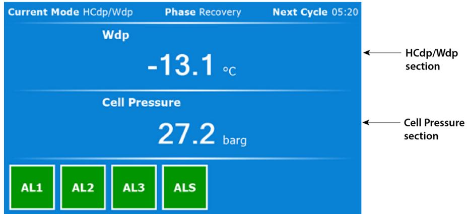
**Figure 12** FRONT PAGE A without External Easidew Fitted
