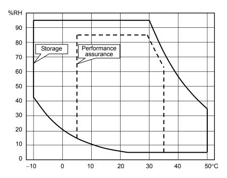
Figure 8-1. Ambient Temperature and Humidity Ranges
