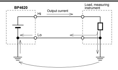
Figure 2-4. Connection to Grounded Load or Measuring Instrument
