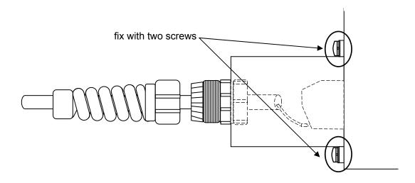
Step4: Tighten the seal nut clockwise with a spanner (20 mm width across flats) with the specified torque of 1.8-2.0 N·m lest the power cable is pulled out.
