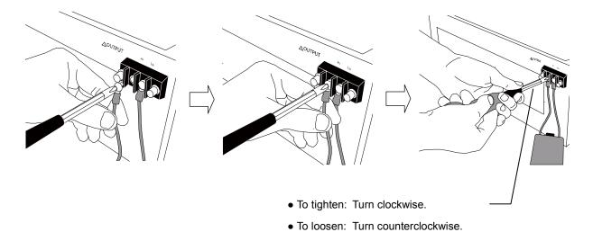
Figure 2-5. Connection to Output Terminals
