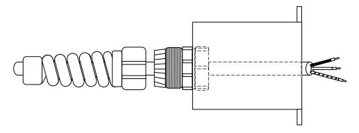
Step2: Loosen the screw on the terminal block using the dedicated driver, open the cable insertion opening as widely as possible, insert the cable core into the opening, and fasten the screw with the specified torque of 1.8 N·m using the dedicated driver.
