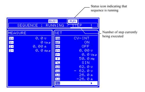
Figure 4-21. LCD Screen When Sequence Is Running
