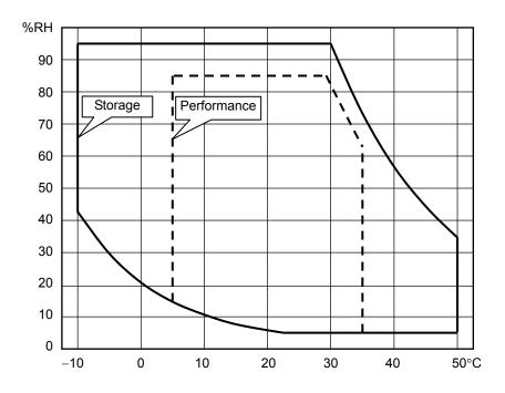
Figure 2-1. Ambient Temperature and Ambient Humidity Ranges
