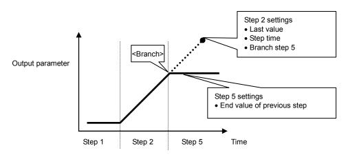
Figure 4-15. Example of Sequence Operation During <Branch>
