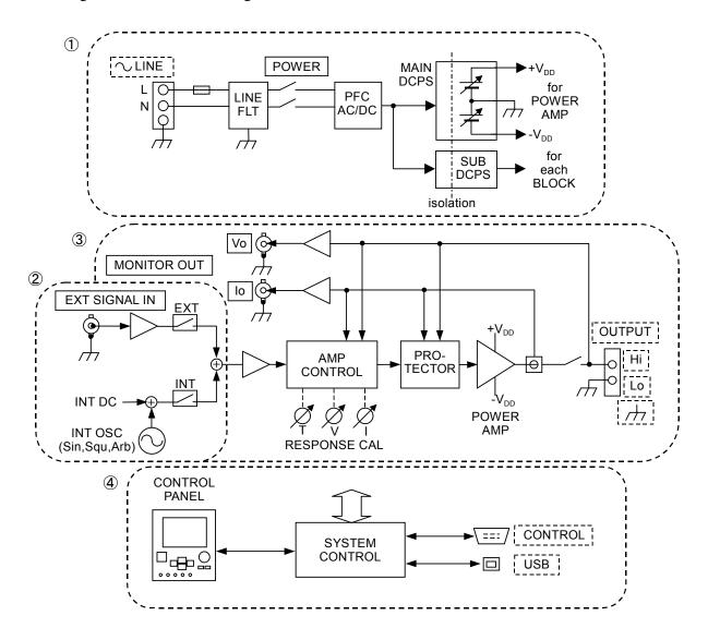
Figure 1-1. Block Diagram
