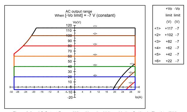
Figure 8-8. AC Output Range (When Negative Voltage Limiter Setting Is Fixed to (7 V)
