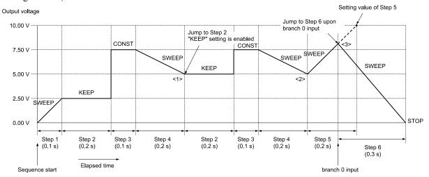
Figure 4-20. Sequence Transition Example (in CV-INT Mode)
