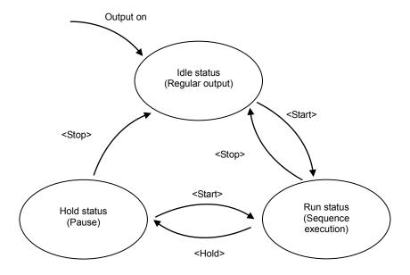
Figure 4-13. Sequence Status Transition Block Diagram
