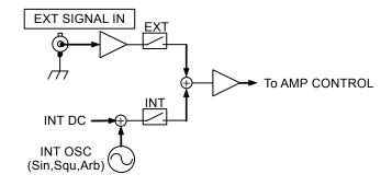
Figure 4-8. Block Diagram of Signal Source Block
