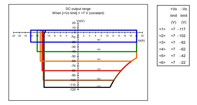
Figure 8-5. DC Output Voltage (When Positive Voltage Limiter Setting Is Fixed to +7 V)
