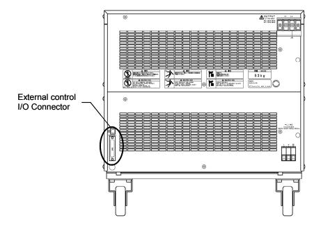
Figure 2-7. External Control I/O Connector
