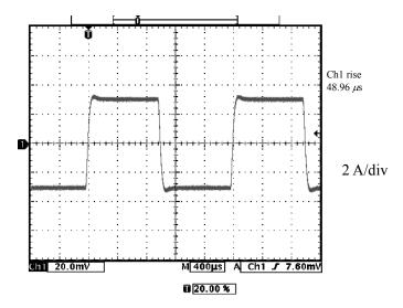
Figure 4-27. Output Current Waveform for CC Mode/Inductive Load (L = 390  $\mu$ H)
