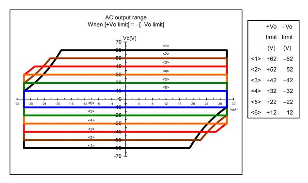
Figure 8-7. AC Output Range (When Positive/Negative Voltage Limiter Settings Are Symmetric)
