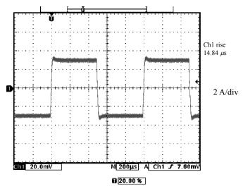
Figure 4-26. Output Current Waveform for CC Mode/Inductive Load (L = 150  $\mu$ H)
