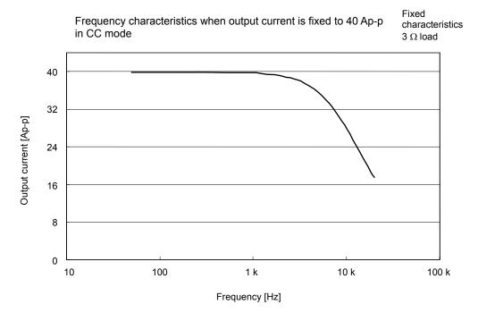
Figure 4-9. Frequency Characteristics for 3  $\Omega$  Load in CV and CC Modes
