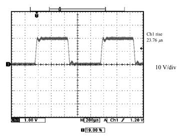
Figure 4-23. Output Voltage Waveform for CV Mode/Capacitive Load (C = 10  $\mu$  F)
