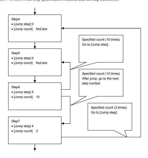
Figure 4-16. Loop Specification Method and Step Transition Example
