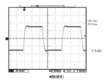
Figure 4-28. Output Current Waveform for CC Mode/Inductive Load (L = 1.6 mH)
