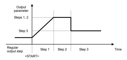
Figure 4-12. Basic Step Transition Example
