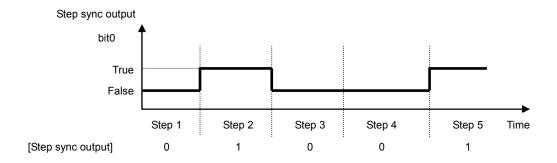
Figure 4-17. Step Sync Output Example
