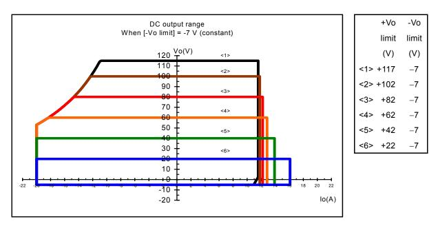
Figure 8-4. DC Output Range (When Negative Voltage Limiter Setting Is Fixed to -7 V)
