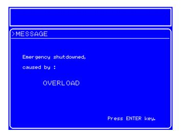
Figure 6-1. Protective Function Related Error Display Examples
