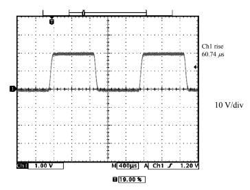
Figure 4-24. Output Voltage Waveform for CV Mode/Capacitive Load (C = 50  $\mu$  F)
