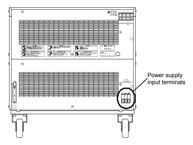
Figure 2-2. Power Supply Input Terminals
