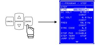
Press the and keys to move the cursor to the digit to be changed and then turn the [MODIFY] dial to set the desired value.
