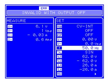
Figure 6-2. Examples of Error Display During Operation
