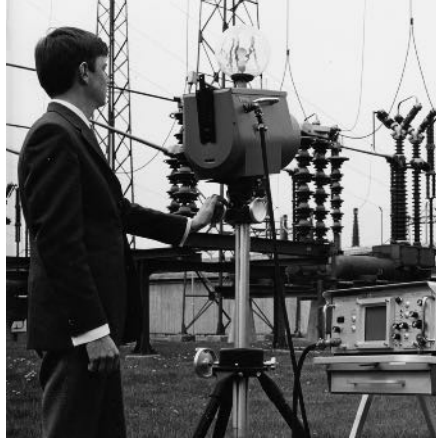
Figure 27.2 1969: Thermovision Model 661. The camera weighed approximately 25 kg (55 lb.), the oscilloscope 20 kg (44 lb.), and the tripod 15 kg (33 lb.). The operator also needed a 220 VAC generator set, and a 10 L (2.6 US gallon) jar with liquid nitrogen. To the left of the oscilloscope the Polaroid attachment (6 kg/13 lb.) can be seen.
