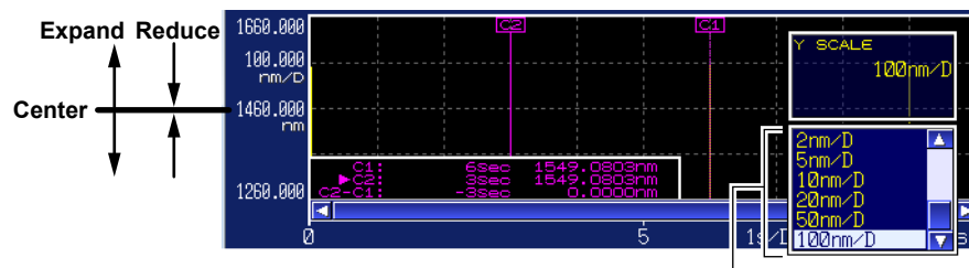
Vertical scale drop-down list box The scale is displayed in 1-2-5 steps.
