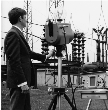
1969: Thermovision Model 661. The camera weighed approximately 25 kg, the oscilloscope 20 kg, and the tripod 15 kg. The operator also needed a 220 VAC generator set, and a 10 L jar with liquid nitrogen. To the left of the oscilloscope the Polaroid attachment (6 kg) can be seen.
