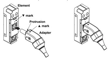
3. Pull lightly on the adapter to make sure that it does not come off.
