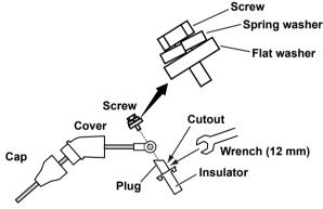
5. Assemble the plug, cover, and cap together.
