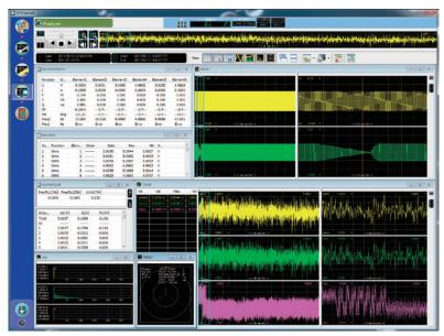
With customizable split screen display of readings in numeric, bar, trend or vector formats, the WTViewerE simplifies the acquisition, storage and analysis of multichannel measurements from up to 4 power analyzers simultaneously.
