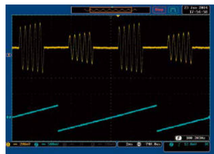
Amplitude modulation of burst oscillation with rising ramp wave
