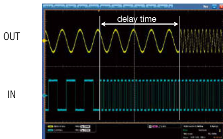
Input of 100 Hz and 500 Hz external signals
