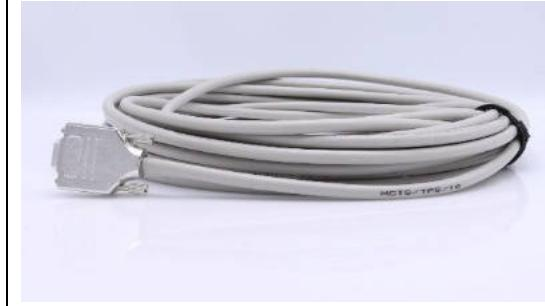
Connection cables from the TPS rack to the transducer are available in various cable lengths. Special cable lengths can be manufactured according demand. Be aware that the cable resistance is part of the maximum measuring resistance. The cables are available with two different wire cross sections, 0.34 mm<sup>2</sup> and 0.75 mm<sup>2</sup>.
