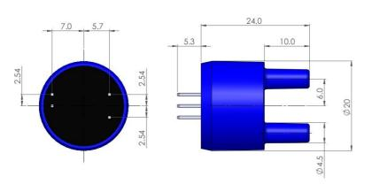
NOTE: 4.5mm OD push-fit tubing connectors.
