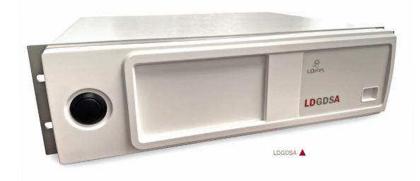
The LDGDSA is a user's friendly gas dilution system that offers all the flexibility to generate automatically the desired gas mixtures. The Windows user's interface gives the ability to control and monitor the mixtures, flows, pressures and the concentrations remotely. The system can store multiple gas cylinder mixtures and it becomes easy to select the right cylinder to generate different blends. It reduces the cost of having specific standard for each blend needed.
