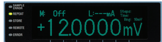
High resolution output with \pm 120000 display counts and 100 nV steps minimum
