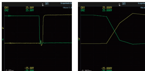
Gate signal waveforms of inverter (20 kHz) The picture on the left shows a waveforms measured with 100 MS/s (by 720211 module) that is sufficiently high sample rate to accurately reconstruct the signal, which will result in more accurate measurements than the one on the right that measured with 1 MS/s
