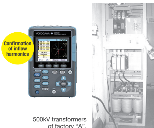
Effect of correspondence: Harmonic contents of 5 th and after dropped and malfunction rate of printing machine decreased.
