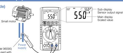
AC/DC clamp-on probe (Model 96095) Reads maximum 60 A when used with the CA450.
