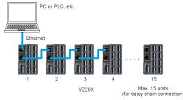
Time synchronization supported in this configuration (daisy chain connection, excluding when Connection type is "1 unit")
