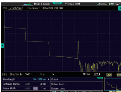
Example of measuring 128-port splitter with high SNR (HSN) mode
