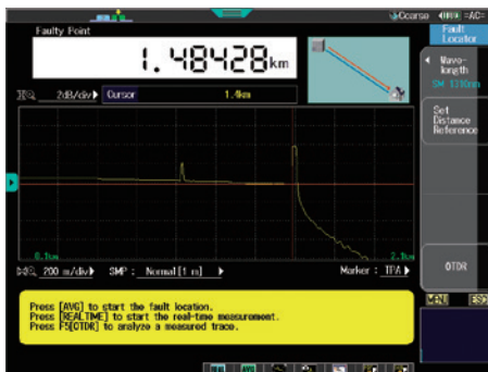
Example of detecting a breaking point 1.48 km away
