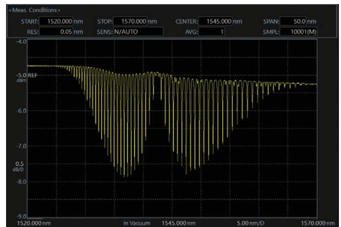
Hydrogen Cyanide \text{H}_{13}\text{C}_{14}\text{N} absorption spectrum measurement with AQ6375E
