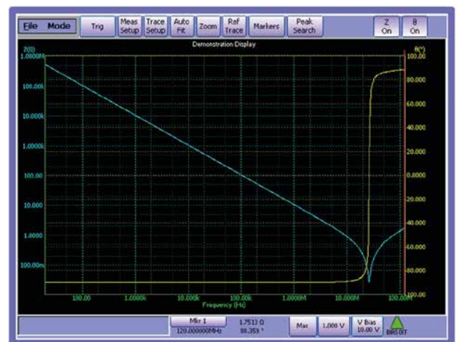
Simultaneous plot of impedance and phase displayed against frequency on a clear colour display
